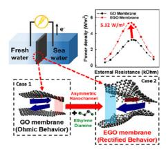
Osmotic power is a sustainable and clean energy source, produced from the salinity gradient between seawater and fresh water. The efficiency of energy generation greatly relies on the performance of ion exchange membranes which govern ion transport behaviors. Nanofluidic channels in lamellar structures have proven to overcome the limit of conventional membranes such as
